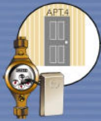
A water meter installed in each apartment is connected to an Inovonics Wireless transmitter.
