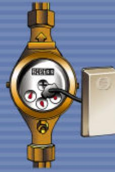
The transmitter then converts the meter read into a digitized signal for transmission.
